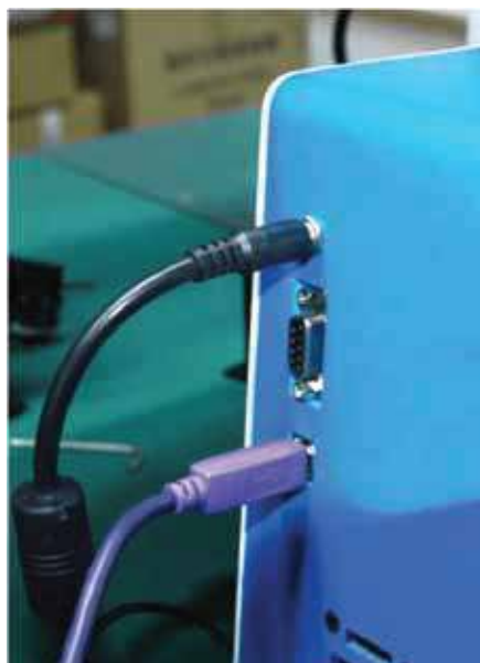
Fig 12 Simple interface: Raman Micro: power socket +USB2.0 connector
