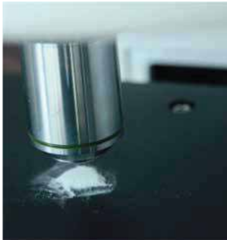
Fig 10 Raman signal high transmission objective, confocal distance length up to 8nm
